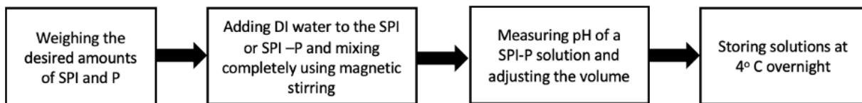
Figure 5.1: Schematic diagram for the preparation of SPI and SPI-Polysaccharide (SPI-P) solution.
