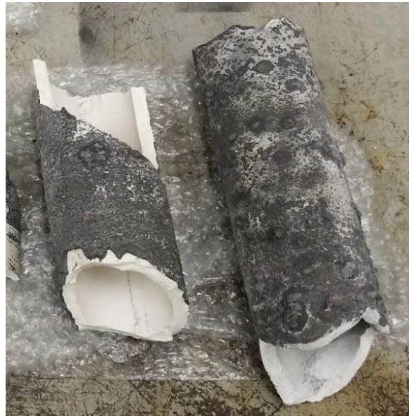
Figure 1-9: Failed furnace rollers covered with aluminum contamination from the Al-Si coating.
