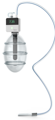
Figure 3.22: Concept design for the first stage pH sensors assembly
