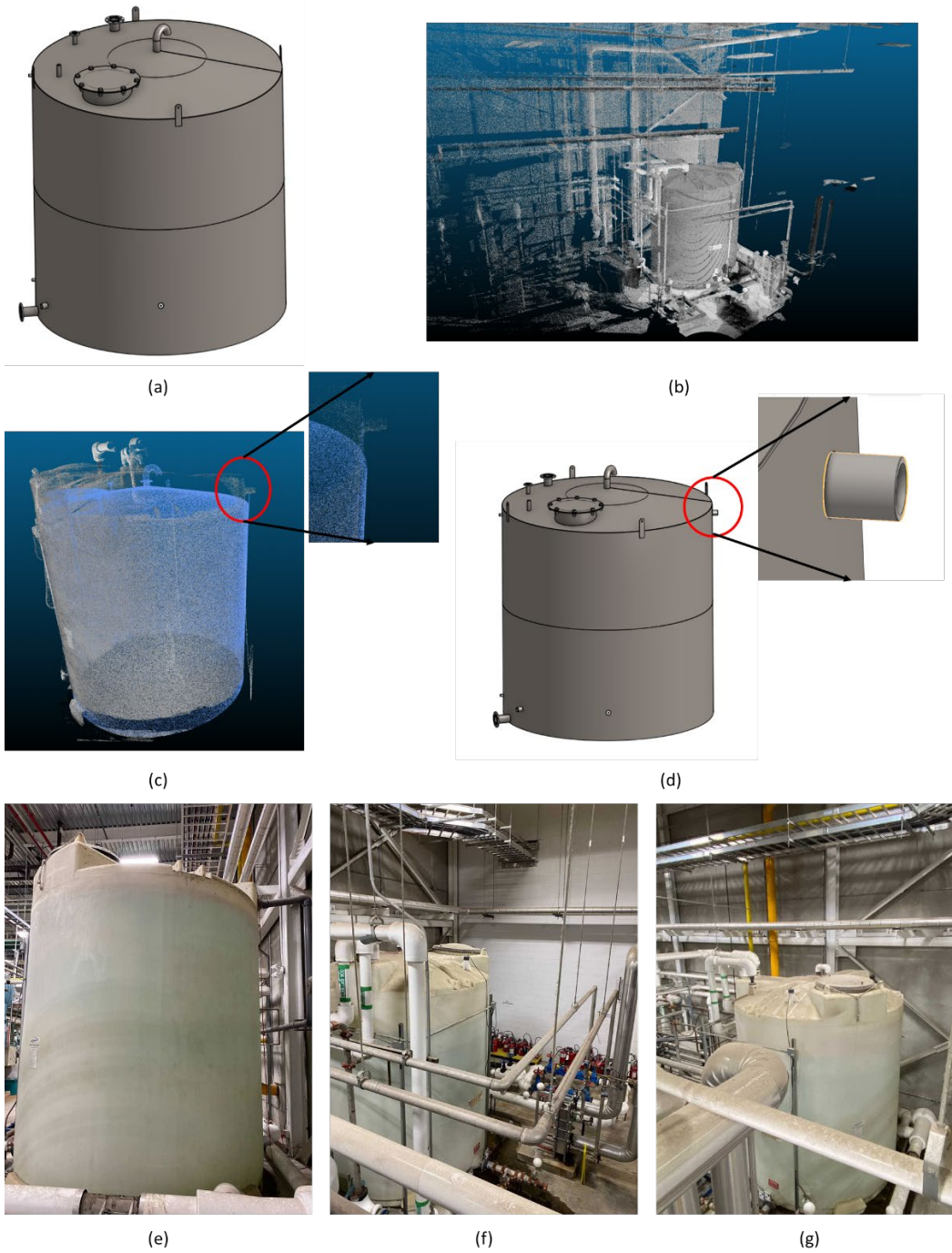
Figure 4-1. (a) Initial design model. (b) The completed site scan of the tank. (c) The scan-vs-BIM reveals a missed nozzle at the back. The blue object is the 3D design model's point cloud and the gray object is the scan point cloud. (d) The missed nozzle was added to the design model. (e) The back nozzle on the existing tank to be replaced by the new tank. (f) Top view of the tank to be replaced. (g) Top view of the tank to be replaced.
