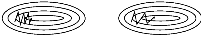
Figure 2.7: SGD without momentum (on the left) and SGD with momentum (on the right) [8]
