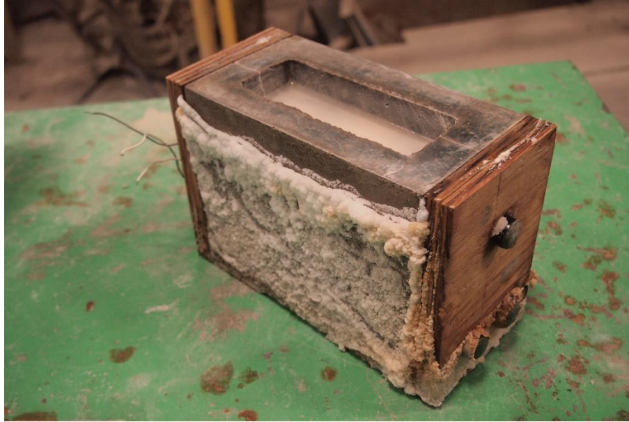
Figure 4-32: Mortar specimen with sodium chloride crystals on surface
