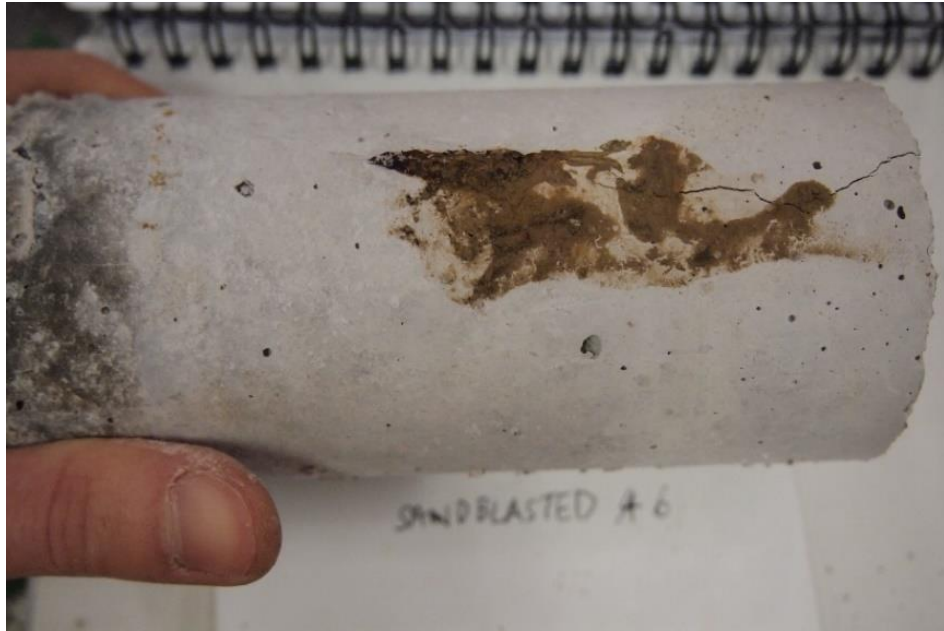
Figure 4-29: Cracked concrete cylinder containing SB06 with rust on surface
