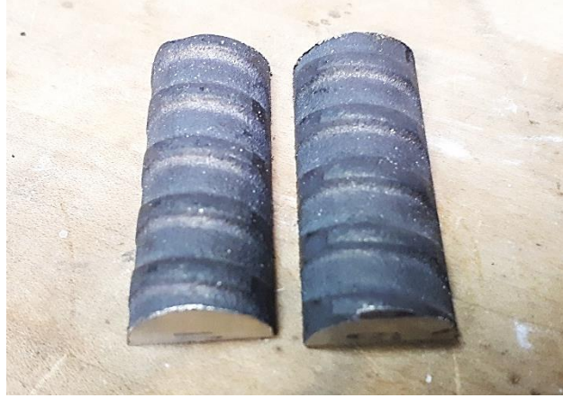
Figure 3-3: Rebar longitudinal sections for microscopy
