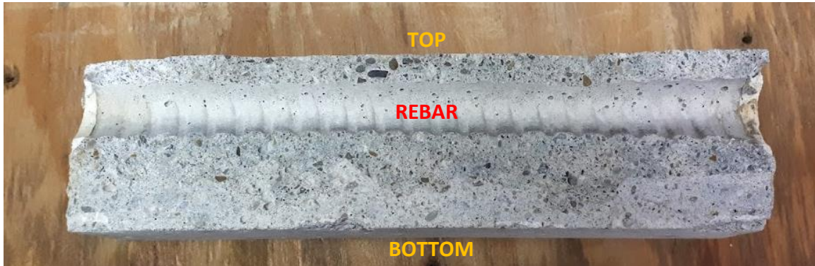
Figure 4-51: Split mortar prism from longer-term corrosion test
