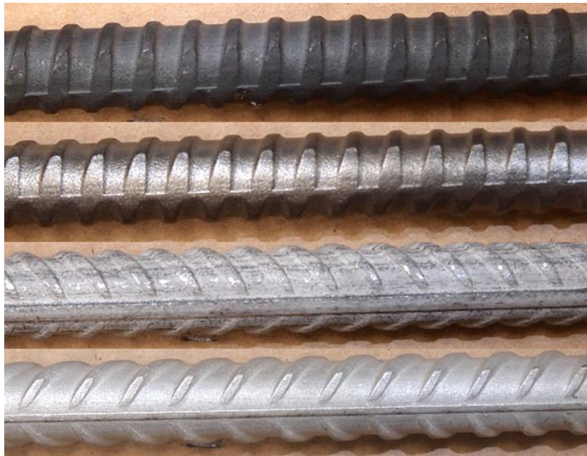
Figure 3-1: Rebar with different surface treatments – (from top) as-rolled, shotblasted-only, pickled-only, pickled-and-shotblasted
