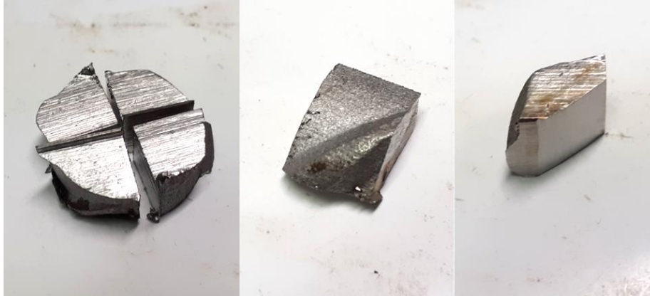
Figure 3-7: (from left) rebar cut into half-hemispheres; top view of curved surface of a single specimen; and isometric of specimen with sharp corner ground flat
