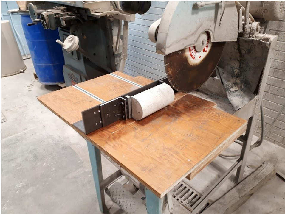
Figure 3-14: Specimen clamp frame for concrete saw, with a concrete cylinder as a cutting sample
