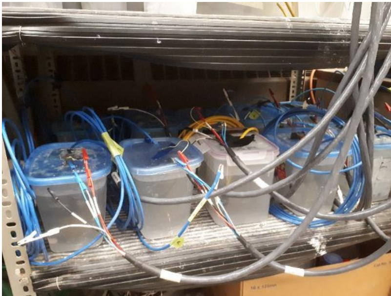
Figure 3-9: Rapid screening test specimens connected to potentiostat
