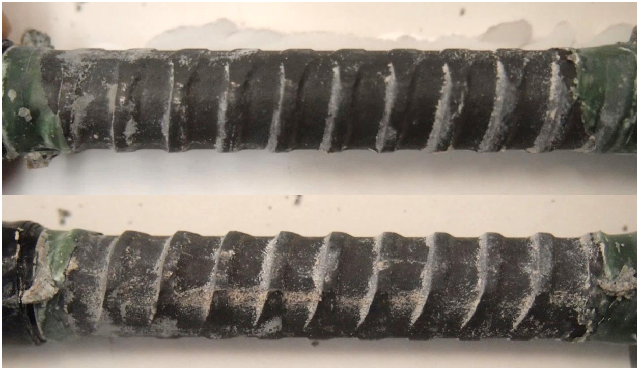
Figure C-2: Specimen AR-04 before testing (top) and after testing (bottom)
