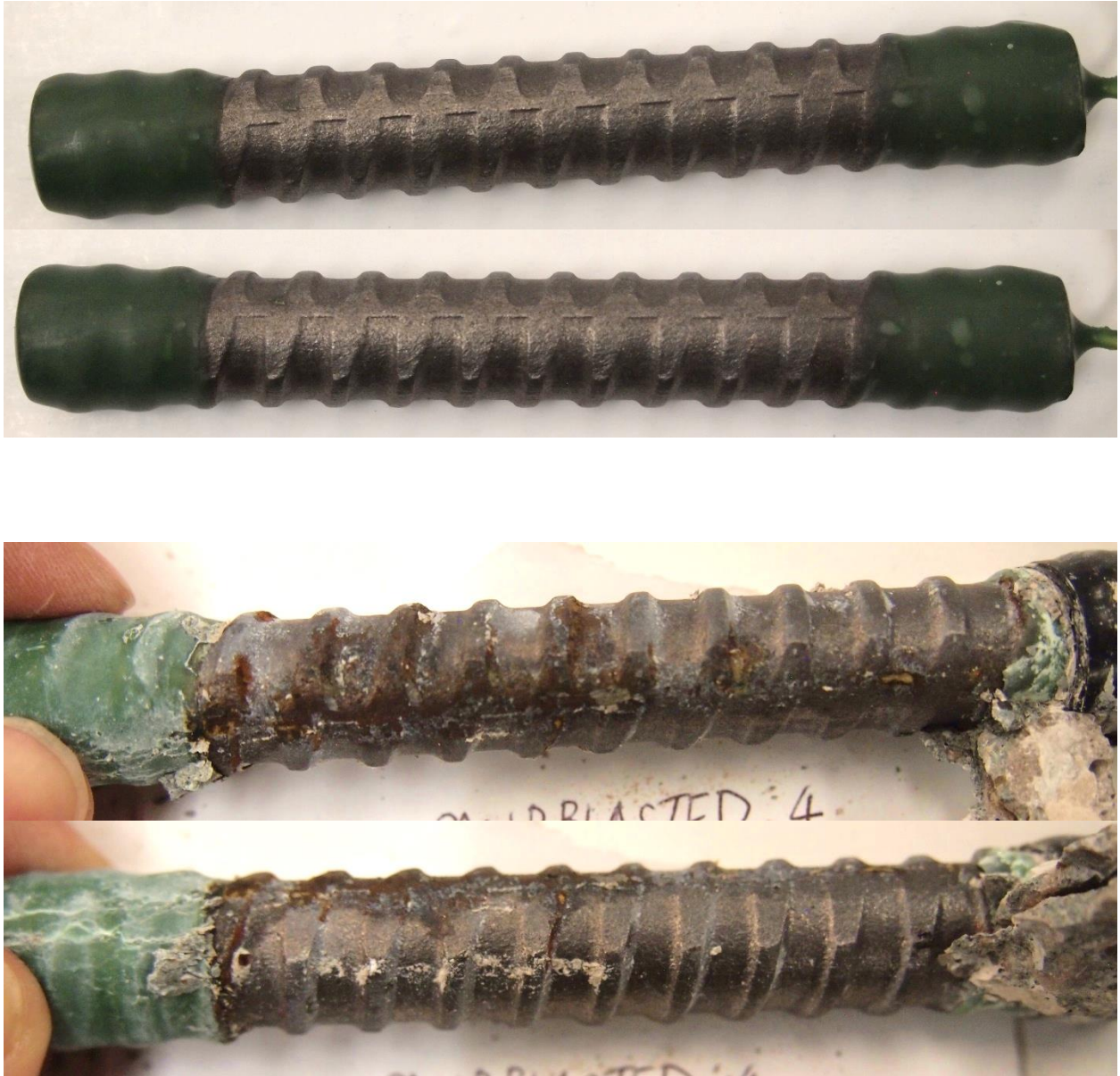
Figure C-18: Specimen SBO-04 before testing (top) and after testing (bottom). Corrosion product observed on rebar surface after testing
