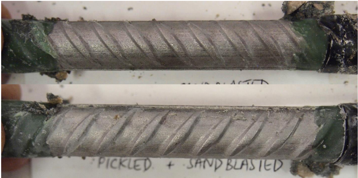
Figure C-12: Specimen PKSB-06 before testing (top) and after testing (bottom)
