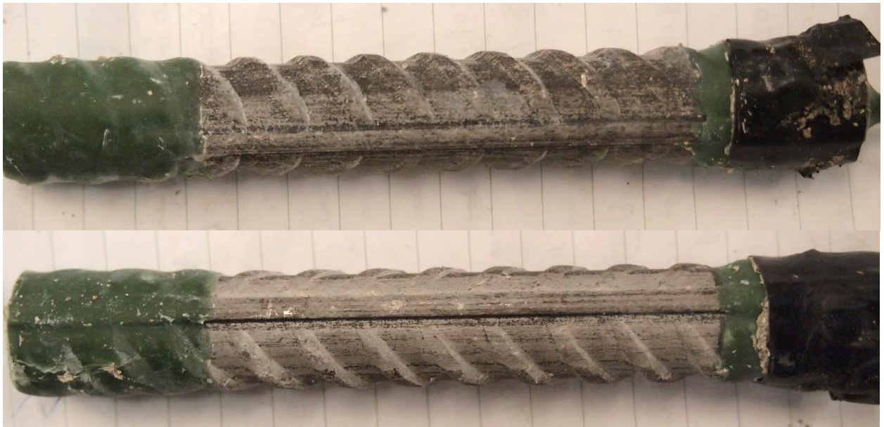
Figure C-6: Specimen PK-04 before testing (top) and after testing (bottom)
