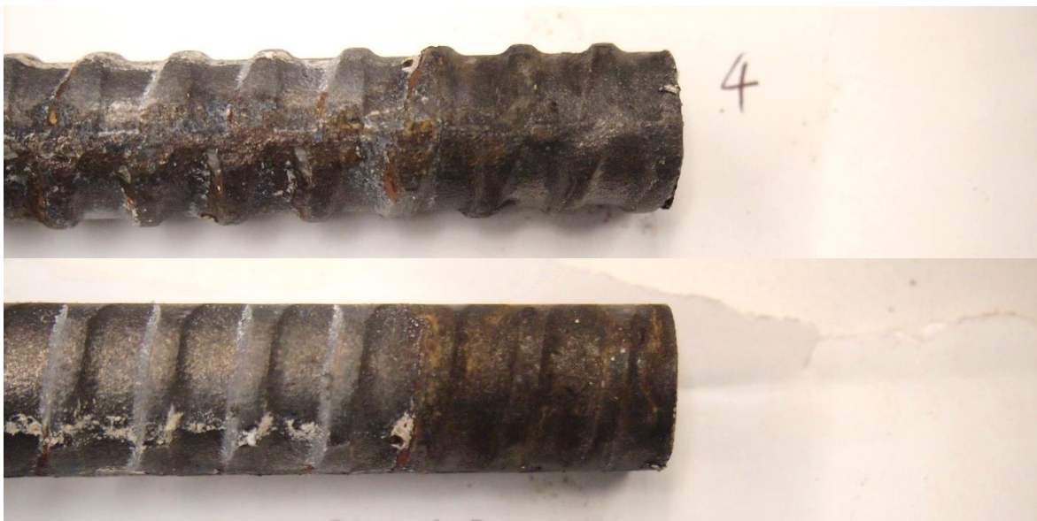
Figure C-20: Corrosion product found under the lacquer at rebar ends on SBO-04 due to crevice corrosion
