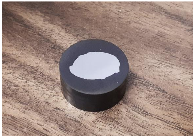
Figure 3-4: Mounted rebar cross-section in resin
