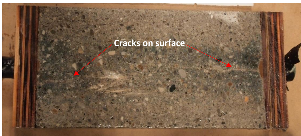
Figure 4-48: Specimen PK-iv with cracks at the bottom of the ponding well. Walls of the well had been removed
