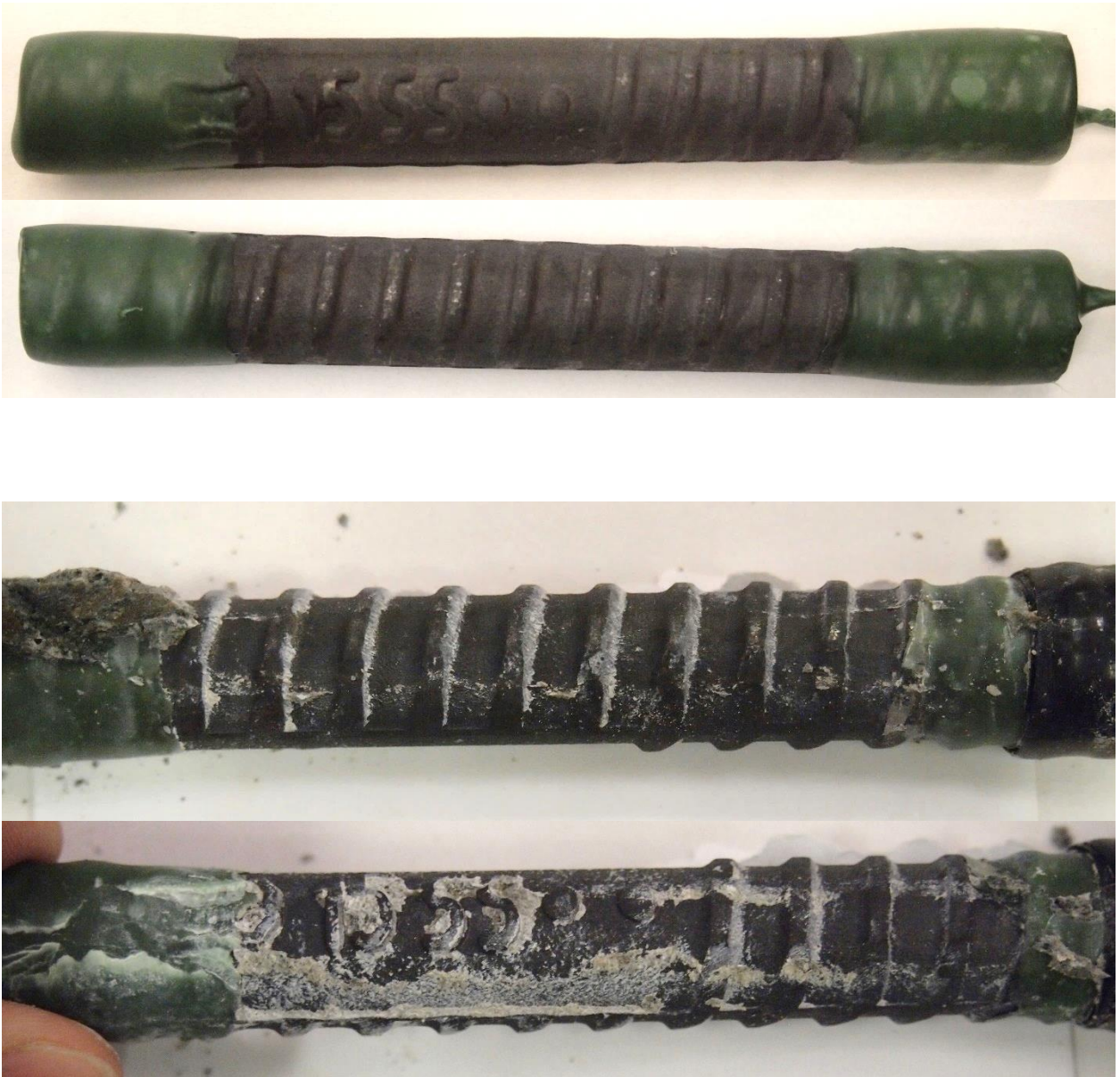
Figure C-1: Specimen AR-03 before testing (top) and after testing (bottom)
