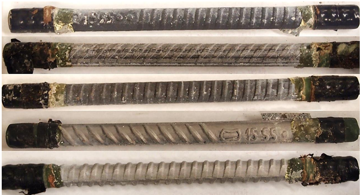
Figure 4-50: Autopsied rebar from mortar specimens. From top: as-rolled, pickled-only, shotblasted-only, shotblasted-and-pickled (classic), shotblasted-and-pickled (threaded)
