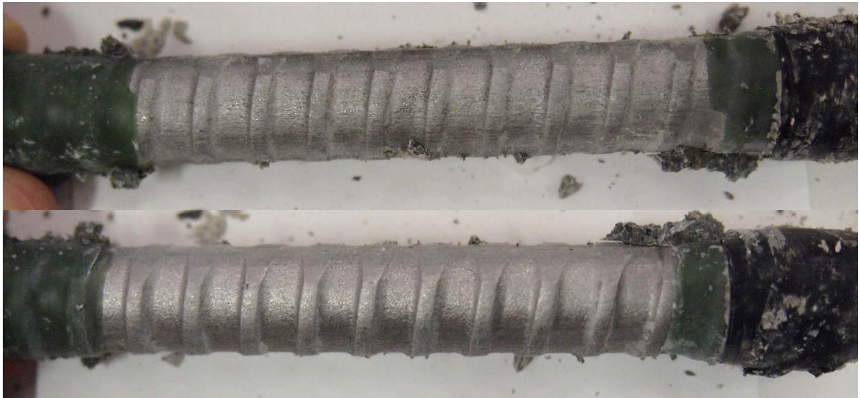
Figure C-15: Specimen PKSBT-05 before testing (top) and after testing (bottom)
