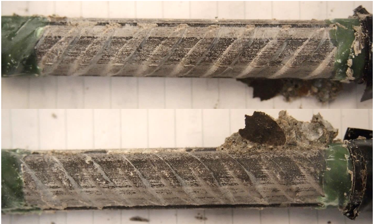
Figure C-5: Specimen PK-03 before testing (top) and after testing (bottom)
