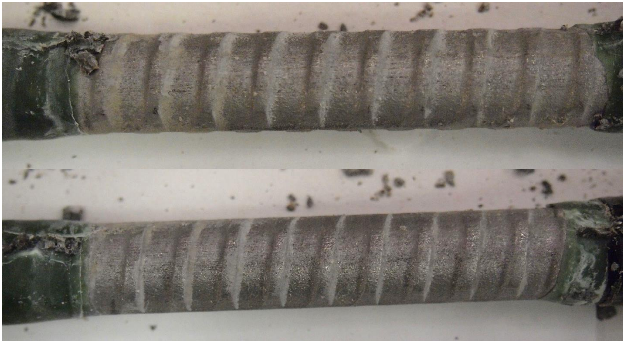
Figure C-13: Specimen PKSBT-03 before testing (top) and after testing (bottom)
