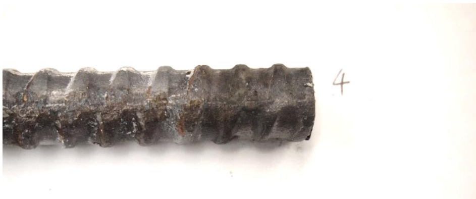
Figure 4-28: Corrosion product found under lacquer at the end of rebar SBO-04
