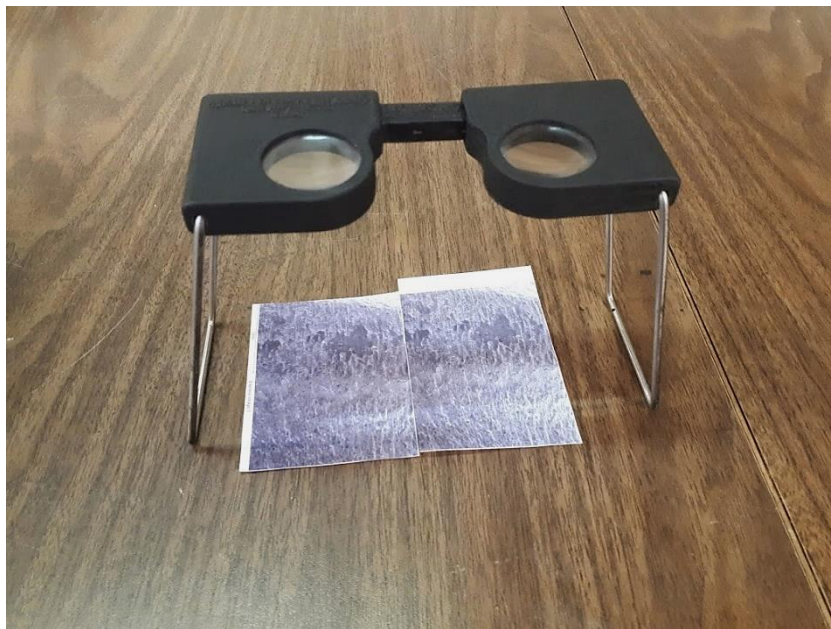
Figure 3-5: Pair of micrographs under a stereoscope
