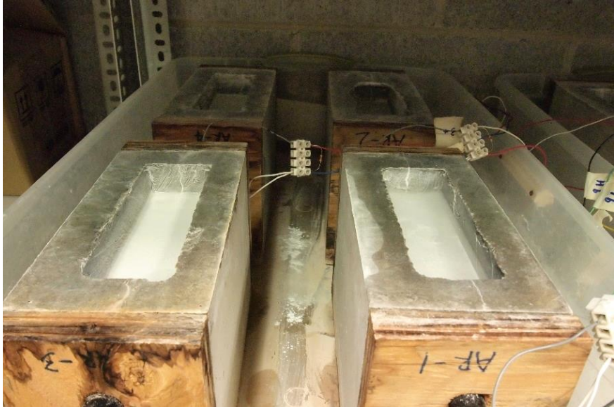
Figure 3-13: Cured mortar specimens connected to resistor
