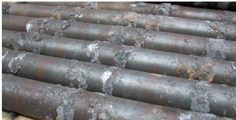
Figure 10: An image showing ceramic rollers heavily damaged by Al-Si coating deposits
