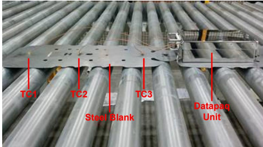
Figure 23: Schematic of Datapaq ® unit attached to a blank.
