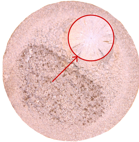
Figure 1.2: A “fisheye” on the carburized axial sample fracture surface
