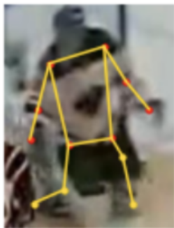
Figure 3.2: An example of a predicted goalie pose using a model with COCO [29] (a large public dataset) pretrained weights. We see that the goalie is on both of his pads, which is a dataset-specific pose that is not common across large public datasets, leading to an incorrect prediction. To achieve acceptable results, more pose annotations of the goalie are required.
