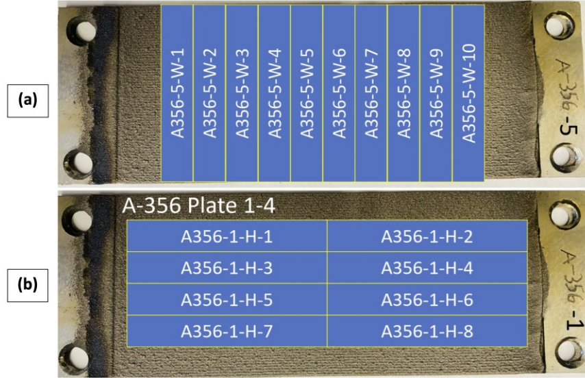
Fig. 18 Diagram of extraction from flat coated plates at two orientations: (a) W-orientation and (b) H-orientation.
