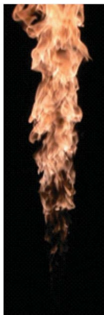
Figure 5.3: Fast-shutter photograph of Sandia ethylene jet flame with Re=20000 . Reproduced from [17]
