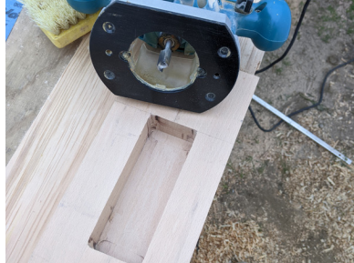
Figure.49 Routing Out the Lamp Base, Photo by Author
