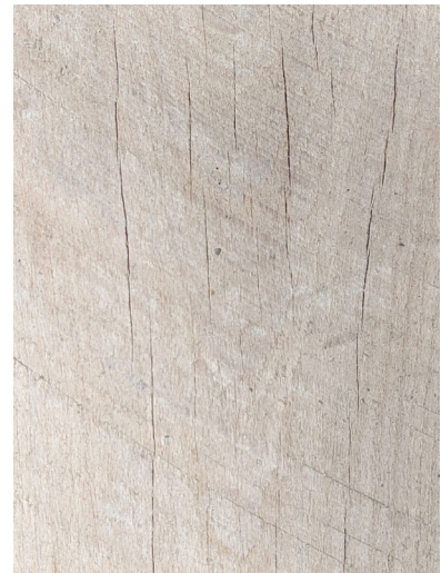
Figure.9 Rough Cut Beech with Surface Checks, Photo by Author
