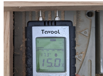
Figure.14 Moisture Meter Reading %15, Photo by Author
