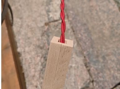
Figure.37 Threading Wire Through Lamp Arm, Photo by Author
