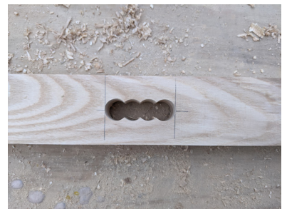
Figure.85 Completed Drilling Sliding desk Component, Photo By Author
