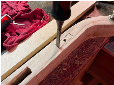
Figure.132 Chiseling Headboard Mortise, Photo by Author
