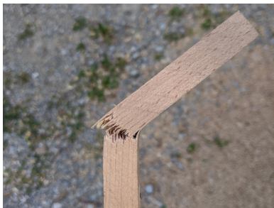
Figure.39 Initial Failed Bend, Photo by Author
