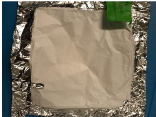
Figure 2-2. Electrospun fibers from PAN on the aluminium foil (as the collector).
