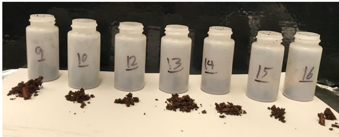
Figure 2-7. Aerogels prepared from heated fibers (when the fibers were initially heated and then cut, the aerogel structure was not formed).
