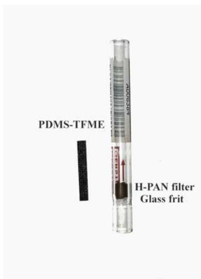
Figure 4-1. PDMS-TFME and H-PAN filter packed inside glass liner.
