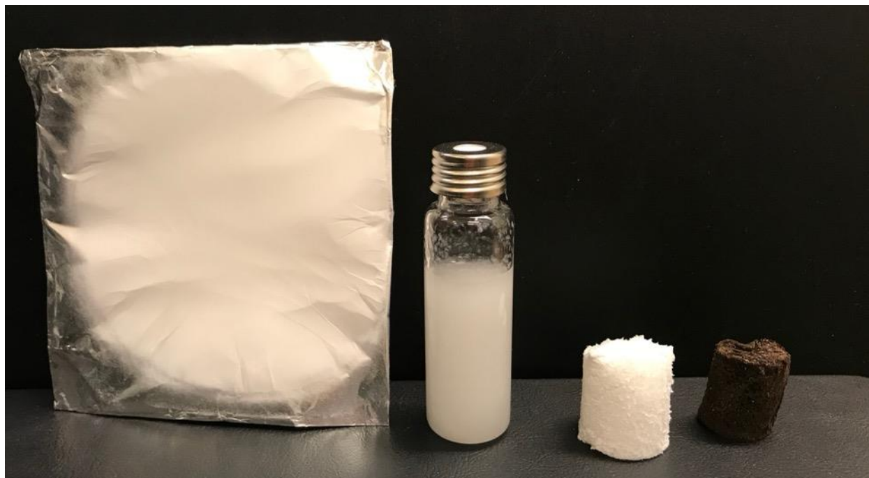
Figure 6-1. The process of preparing filter, from left to right, electrospun fiber, fiber-water suspension, PAN aerogel (white) and heated PAH (H-PAN) aerogel (brown)
