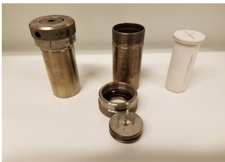
Figure 2. 1: Teflon container (right), steel autoclave (middle) and fully setup reaction vessel (left).
