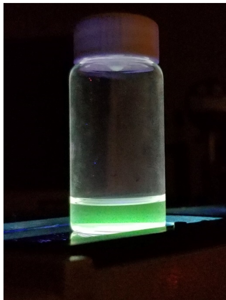
Figure 3. 19: Image of green emitting Tb-CNPs in colloidal suspension in hexane, under near UV excitation
