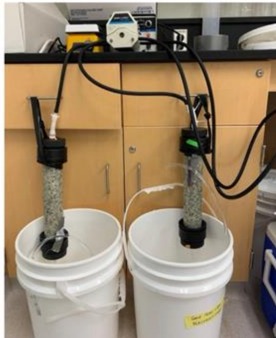
Figure D - 2 A) Mixing of wildfire ash and raw Grand River water to create low (two leftmost beakers), moderate (two middle beakers), and high (two rightmost beakers) ash content water. B) Roughing filtration pre-treatment set-up. Influent is controlled with peristaltic pump pictured here on lab bench.
