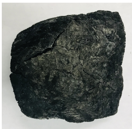
Figure 3.19: The state of the oriented strand board sample post exposure to 25 kW/m 2 incident heat flux in the cone calorimeter
