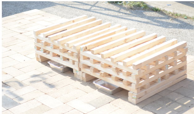
Figure 4.7: Two wood cribs placed side by side representing a 500 kW design fire
