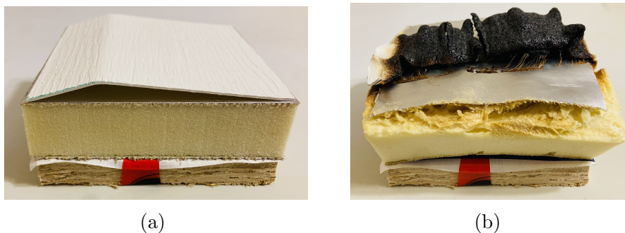
Figure 3.25: The state of Sandwich #2 samples (a) before and (b) after exposure to 15 kW/m 2 external incident heat flux in the cone calorimeter
