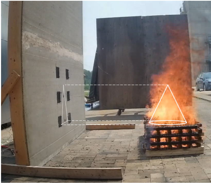
Figure 4.20: The design fire plume core and its projection onto the exposed wall surface
