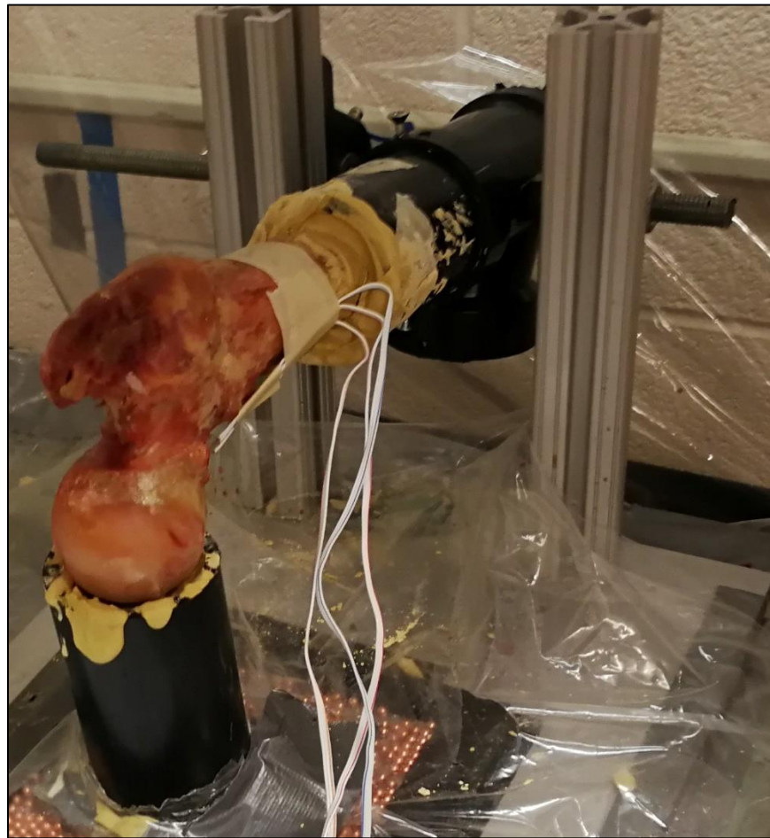
Figure 4-2: Proximal femur specimen mounted in the mounting jig. The jig was affixed to the top surface of the force plate and placed beneath the load carriage of the vertical drop tower Hip Impact Simulator (HIS).
