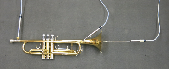
Figure 1: (Colour online) Placement of microphones on the Barcelona BTR-200LQ trumpet.
