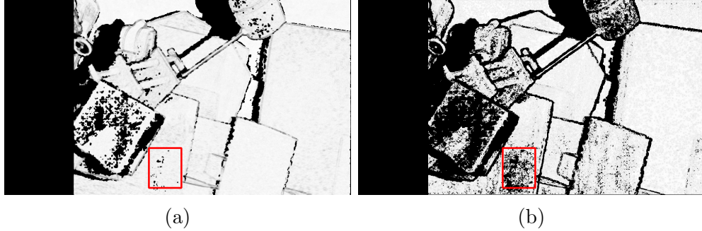
Figure 4.7: Confidence maps computed by (a) ZSAD only and by (b) the proposed method. The red rectangle outlines a textureless region from the RGB image in Figure 4.3.
