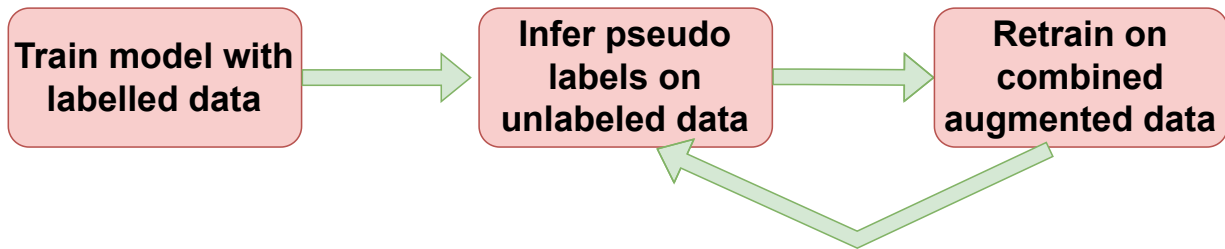
Figure 7.2: General pseudo labelling technique for semi supervised learning. A model is first trained on limited labeled data, which is used to infer labels on unlabeled data. Then the model is re-trained on combined data with data augmentations applied. The process is repeated in cyclic manner to obtain acceptable results.
