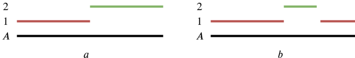
Figure A.1: Motivation for ID-based measures. CLEAR MOT metrics charge one identity switch error to (a) and two identity switch errors to (b). However applications such as sports player tracking favour (b) instead of (a) since (b) maintains the identity for a longer time.
