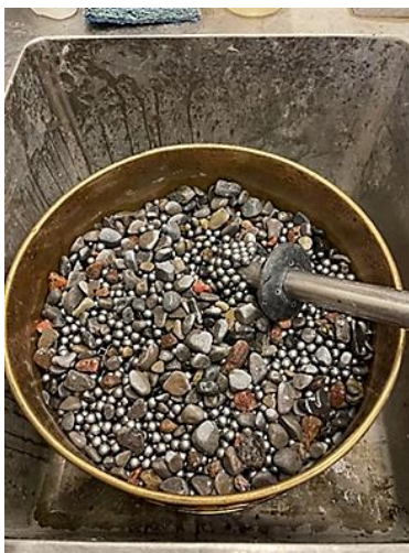
Figure 3-15 Steel balls being separated from aggregates using magnetic rod after Micro-Deval abrasion test
