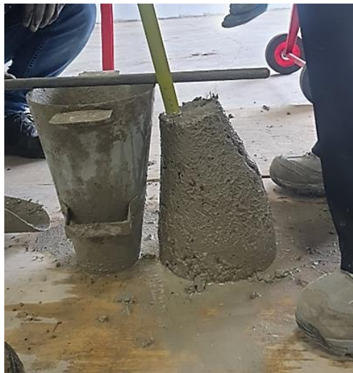
Figure 3-17 Measurement of the slump in fresh concrete
