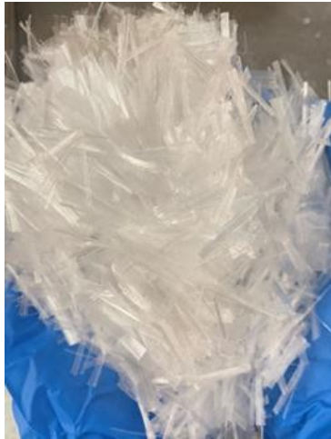
Figure 3-9 Micro synthetic fibre used in this study
