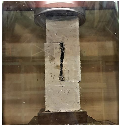
Figure 4-7 Specimen after undergoing shear test
