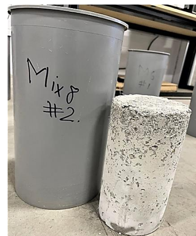
d. RC 40/S 20/G 10 mix after 28 freeze-thaw cycles
