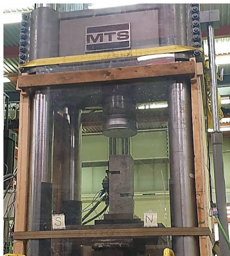
Figure 3-20 Shear strength test setup
