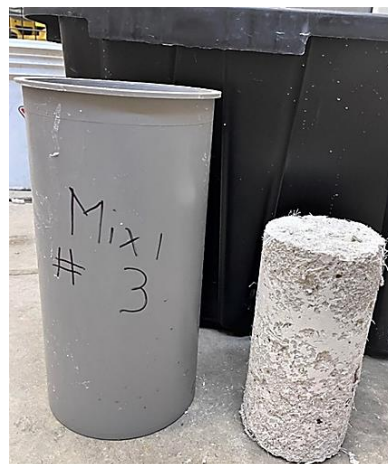
b. RC 20 mix after 28 freeze-thaw cycles
