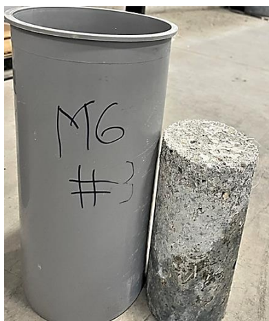
c. RC 20/S 20 mix after 28 freeze-thaw cycles
