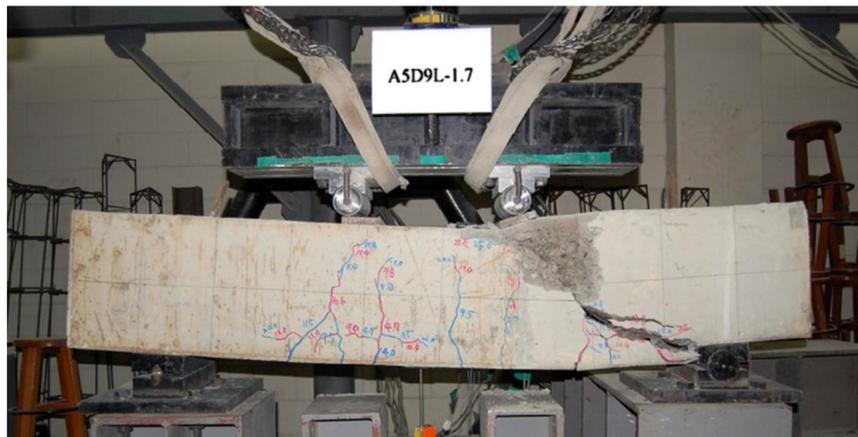
**Figure 3.5: Typical failure pattern of beams tested by D. J. Kim et al. (2014)**
