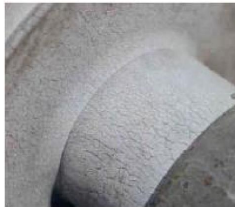
Figure 7. Crazing seen on non-ceramic insulators [8]
