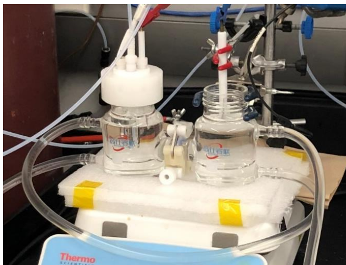
Figure 14. Photo of the experimental set-up for the locally encapsulated BCA promoted electrochemical bicarbonate utilization system configuration. The cathodic compartment on the left comprises the Ar saturated 0.5 M \text{KHCO}_3 electrolyte along with the encapsulated BCA containing Au BNPs working electrode, and the Ag/AgCl reference electrode which are connected to the potentiostat through the red and white alligator clips, respectively. The Nafion CEM separates the cathodic compartment from the anodic compartment on the right which contains the Pt mesh counter electrode that is connected to the potentiostat through the blue alligator clip. The electrolyte in this compartment is also 0.5 M \text{KHCO}_3 .
