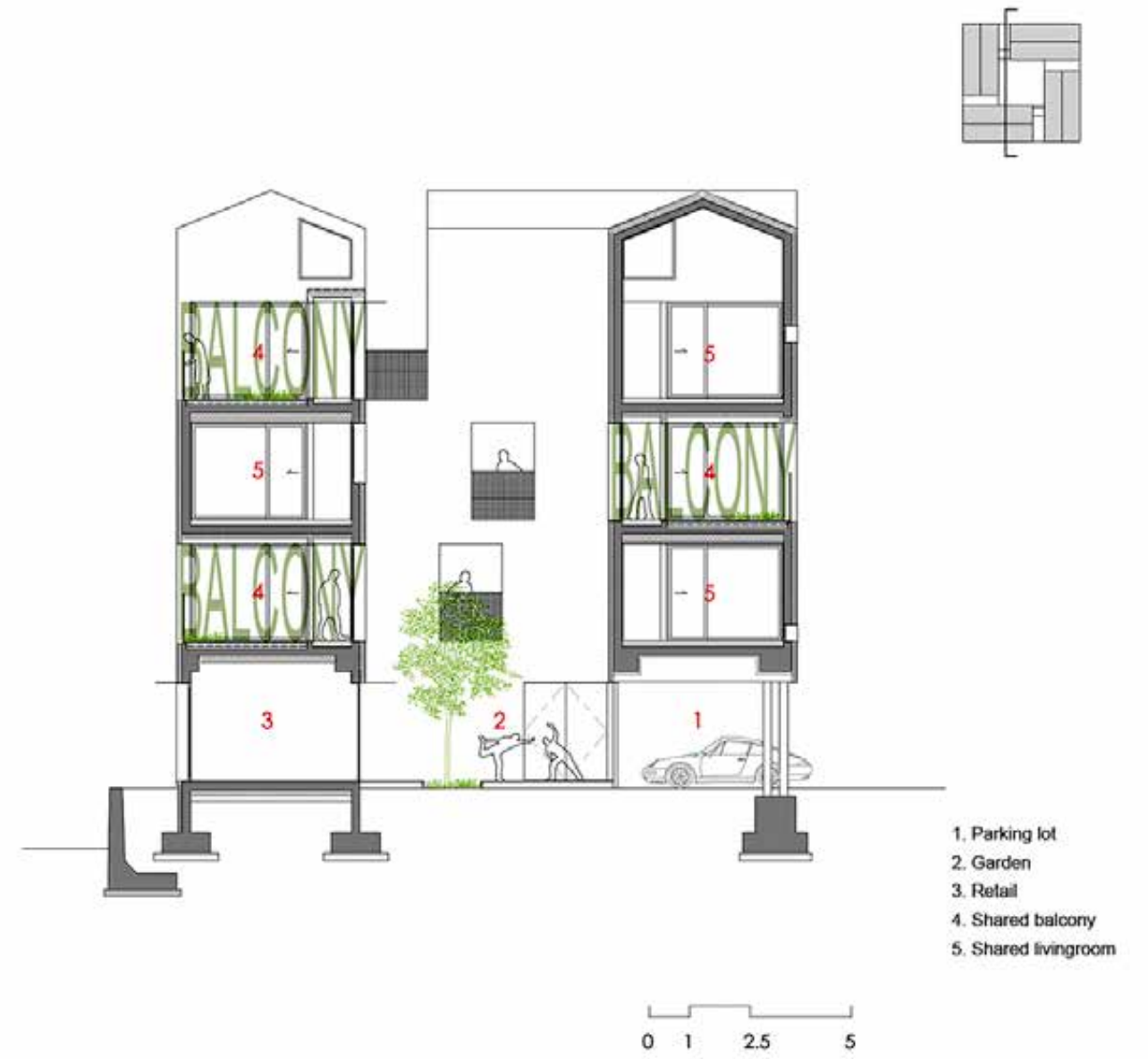
Fig. 4.46 Gap House Section
