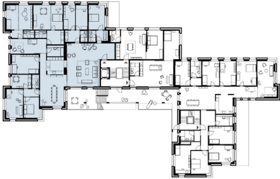
Fig. 4.7 Heizenholz Floorplan Cluster Apartment Unit
