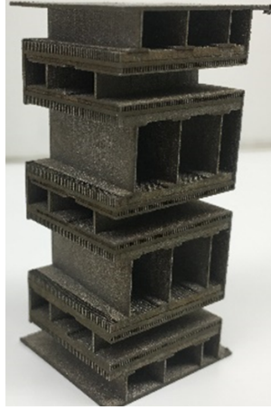
Figure 3.11: Cut view of 2" x 2" x 2" MMHX (Fig. 3.5(b))
