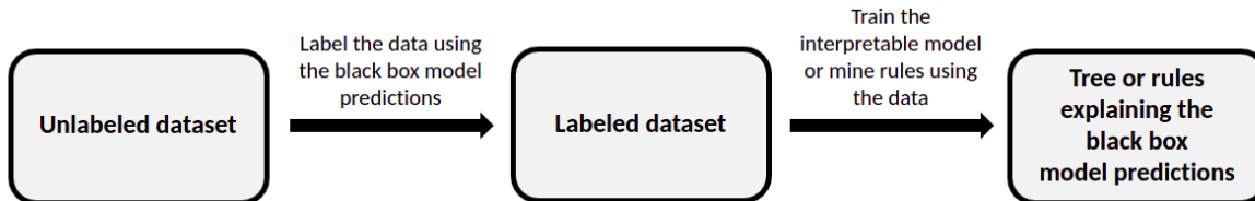
Figure 1.3: General process of the surrogate approach for explaining black box models using interpretable methods
