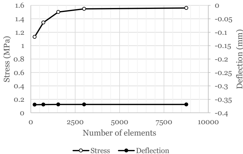
Figure 3.25: Number of elements used in the slab versus the observed maximum stress and deflection in the slab
