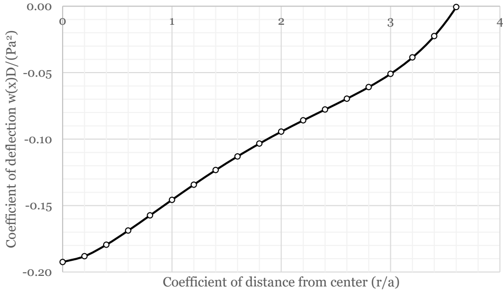
Figure 2.29: Deflection profiles for an infinite plate resting on an elastic half-space subject to a concentrated load, produced by Hogg’s (1938) equations
