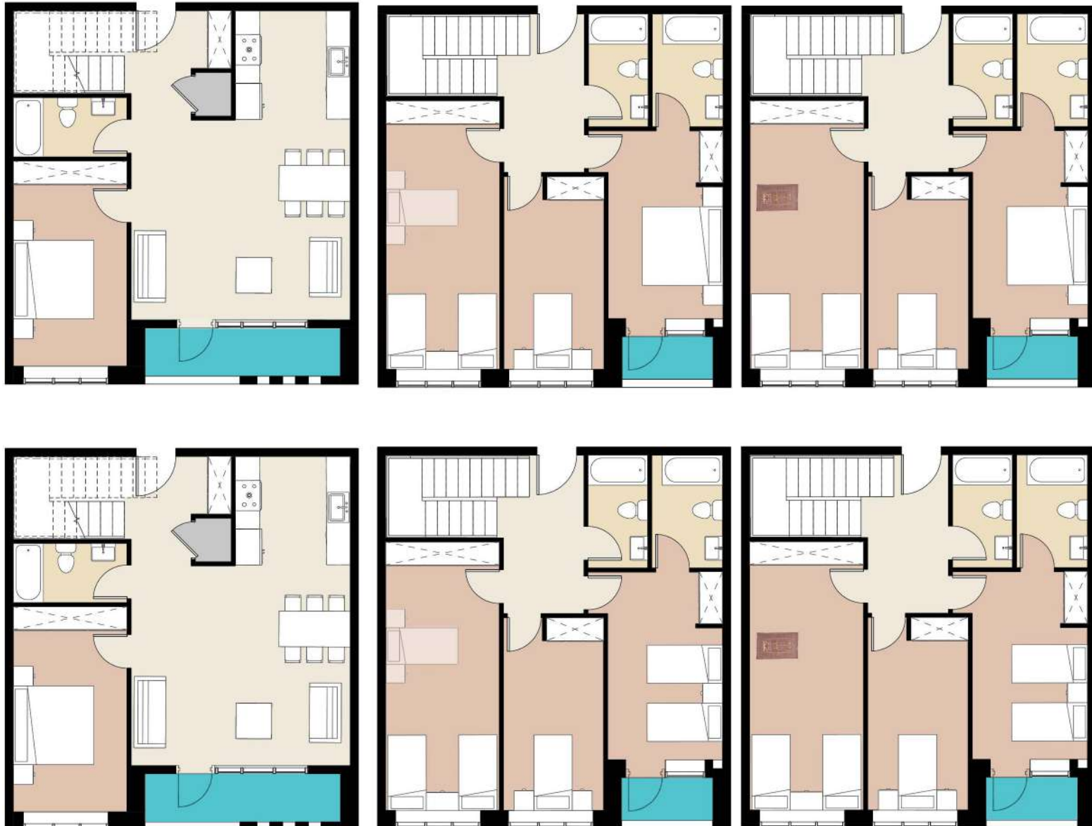
Fig3.47. Big Family unit with the possibility of adding one bed and individual prayer space.
