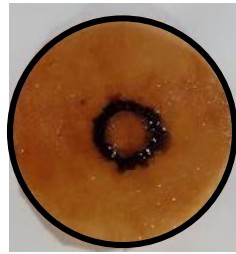
Figure 4.29: Aged (300 hours) paper under repetitive transient voltage of amplitude = 6 kV, switching frequency = 1 kHz, duty cycle = 50%, and rise time = 220 ns with Voltesso 35 A oil.
