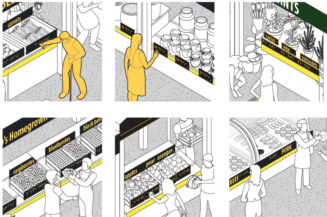
Figure 6.5 Information on product types, prices displayed on product boxes, display table edges through braille, high contrast labels and materiality
