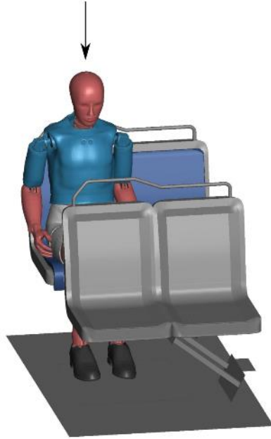
Figure 85: Inboard and outboard seating locations in the test buck model
