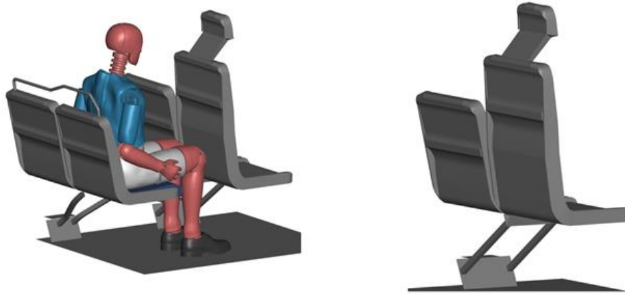
Figure 89: Forward seat with headrest and raised seatback
