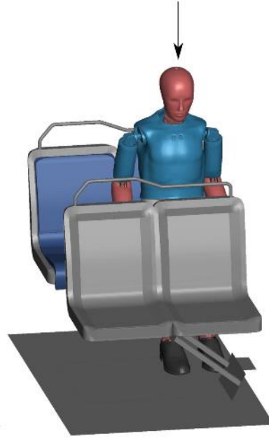
Figure 85: Inboard and outboard seating locations in the test buck model
