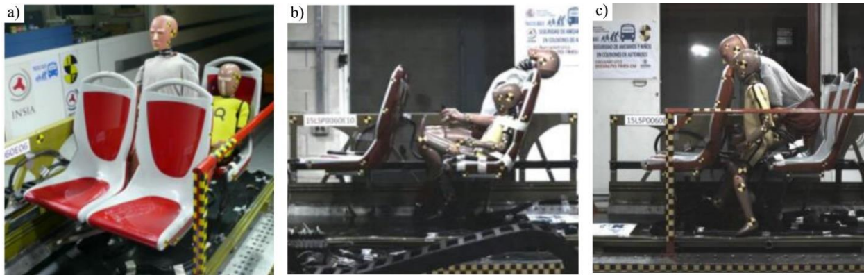
Figure 48: a) Test buck with HIII 50 th percentile ATD and 6 YO ATD; b) Rear impact hyperextension of neck due to low seat back; c) Face of ATDs impact the top of the forward seat in the frontal impact (Copyright Permission [119])
