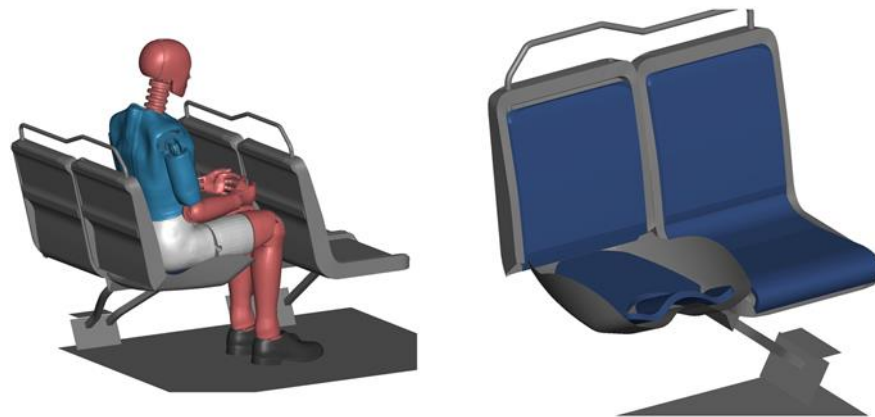
Figure 88: Raised lip on seat pan to limit the forward sliding of the passenger
