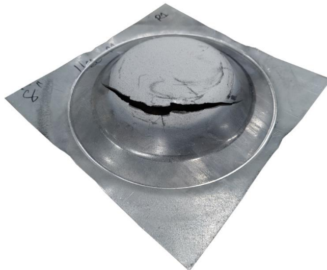
Figure 16: Radius fracture that occurred in the Marciniak test for 3rd Gen 1180 V1
