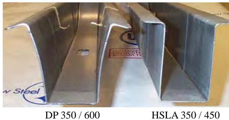
Figure 11: Comparison of springback for DP steel and HSLA (World Auto Steel, 2019)
