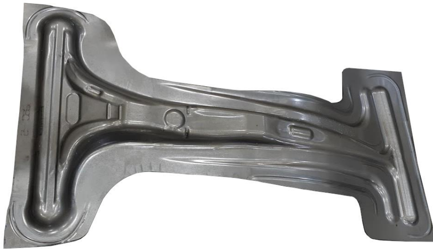
Figure 76: A successful forming trial of the 3rd Gen 980 B-pillar
