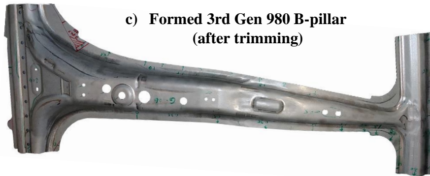
Figure 68: B-pillar CAD geometry a) before trimming used in tooling design, b) a formed 3rd Gen 980 B-pillar before trimming indicating the locations of the side sill, fold initiators, and roof rail and c) a formed 3rd Gen 980 B-pillar after trimming
