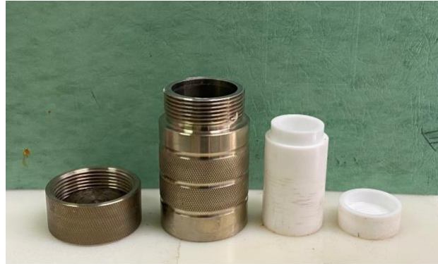
Figure 3-6. The autoclave parts and the cylindrical Teflon
