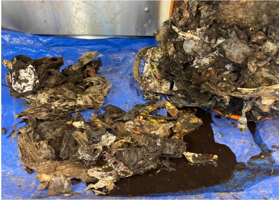
Figure 3.1. Excavated Waste Residue (EWR) from Calgary Bio-cell
