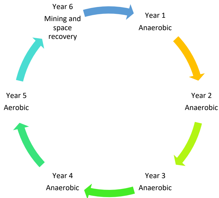
Figure 1.2. Phases of bio-cell operation with example durations [23]
