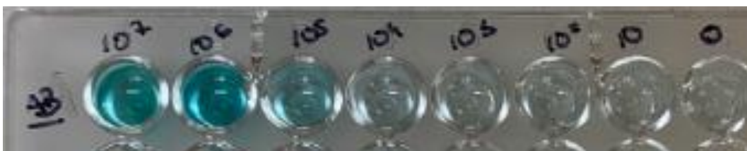
Figure 8. Visual limit of detection for live Cryptosporidium using HRP-labelled antibodies. A blue color indicating the presence of oocysts is shown.
