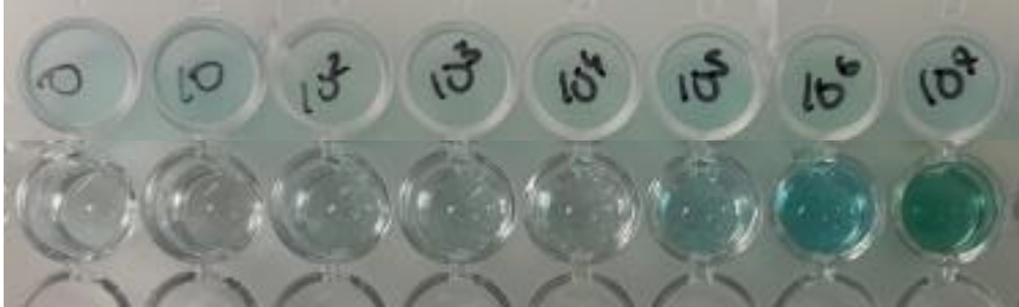
Figure 12. Visual limit of detection for heat-inactivated Cryptosporidium using HRP-labelled antibodies. A blue color indicating the presence of oocysts is shown.
