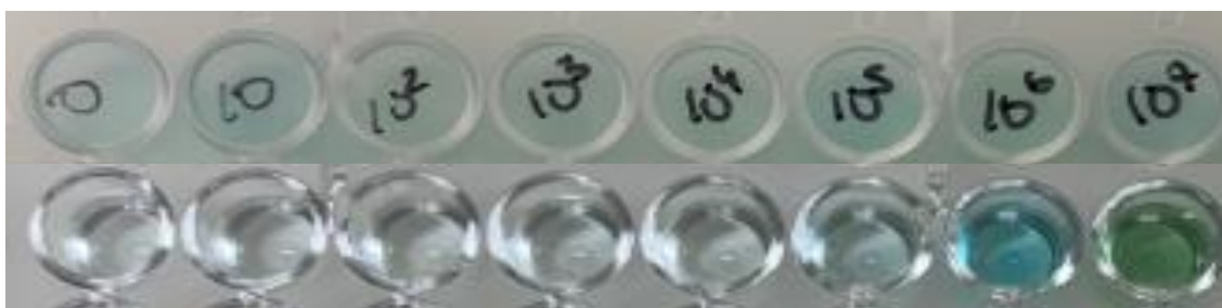
Figure 14. Visual limit of detection for freeze-inactivated Cryptosporidium using HRP-labelled antibodies. A blue color indicating the presence of oocysts is shown.
