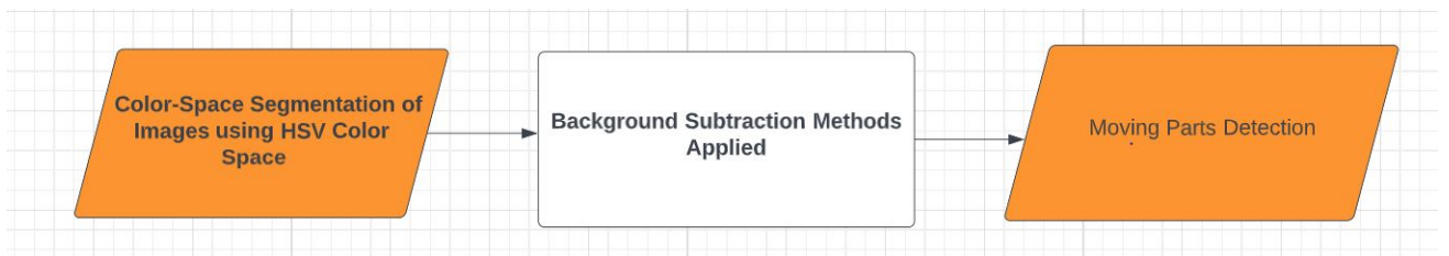
Figure 4.1: Overview of performing and evaluating color-space segmentation through moving parts detection in assembly machines
