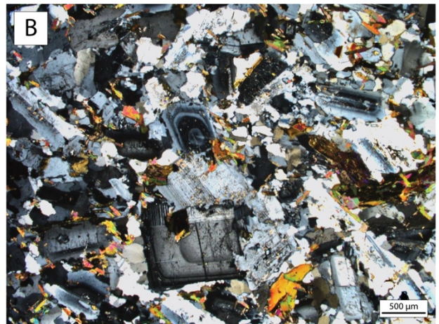
Figure 8: Photomicrographs of granodiorite: (A) Inequigranular with myrmekite texture. (B) Inequigranular with coarse zoned plagioclase.
