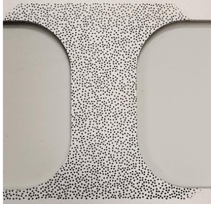
Figure 58: Example of speckled LDH specimen for DIC strain measurement [130].
