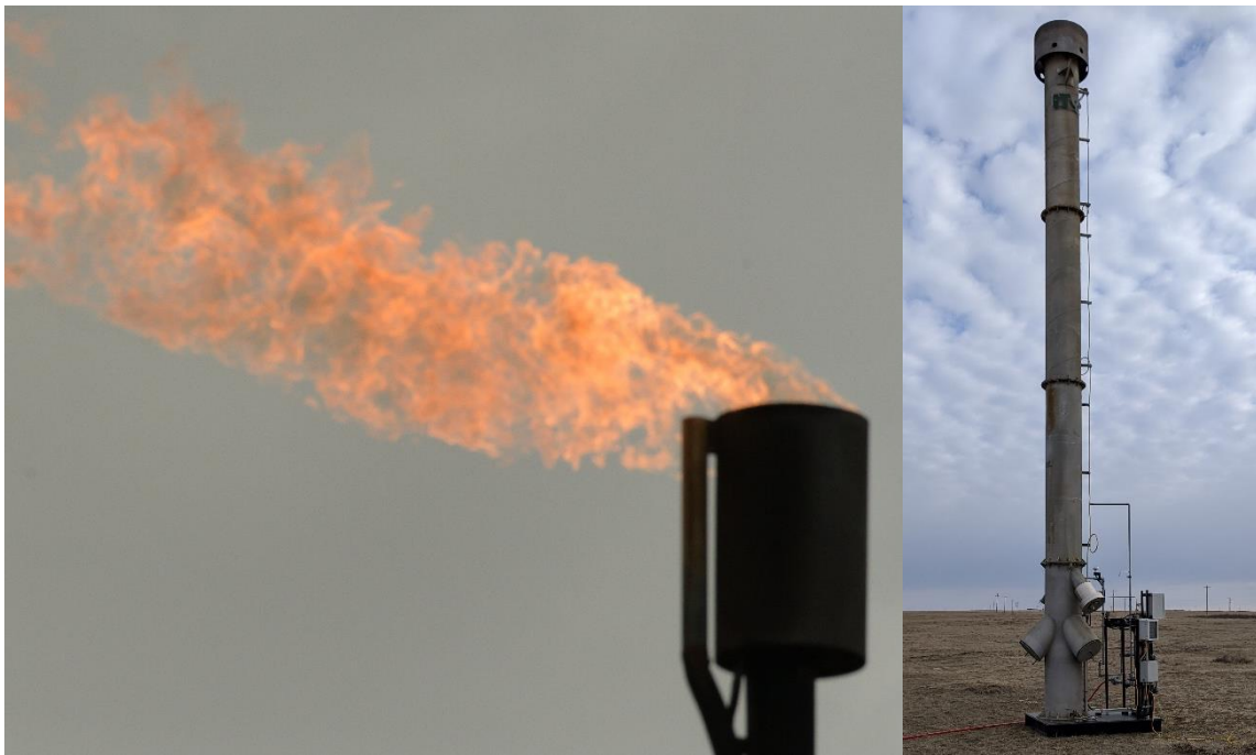
Figure 40: Alberta field measurements (left) methane release into lit flare (right) combustor
