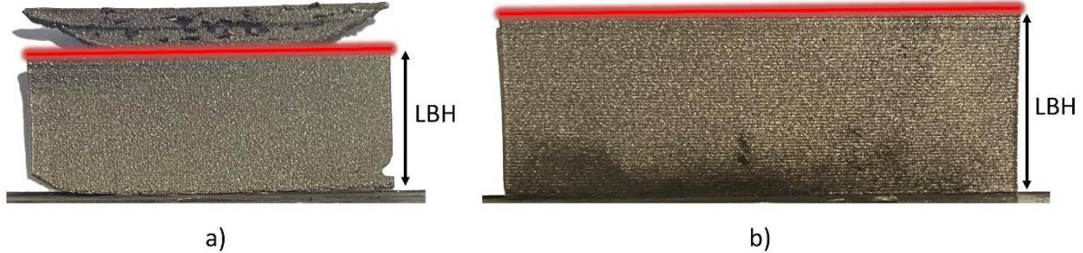
Figure 8-3: LBH measurement criteria for a) partial and b) complete part failure. The red lines indicate the end positions of the LBH measurements.
