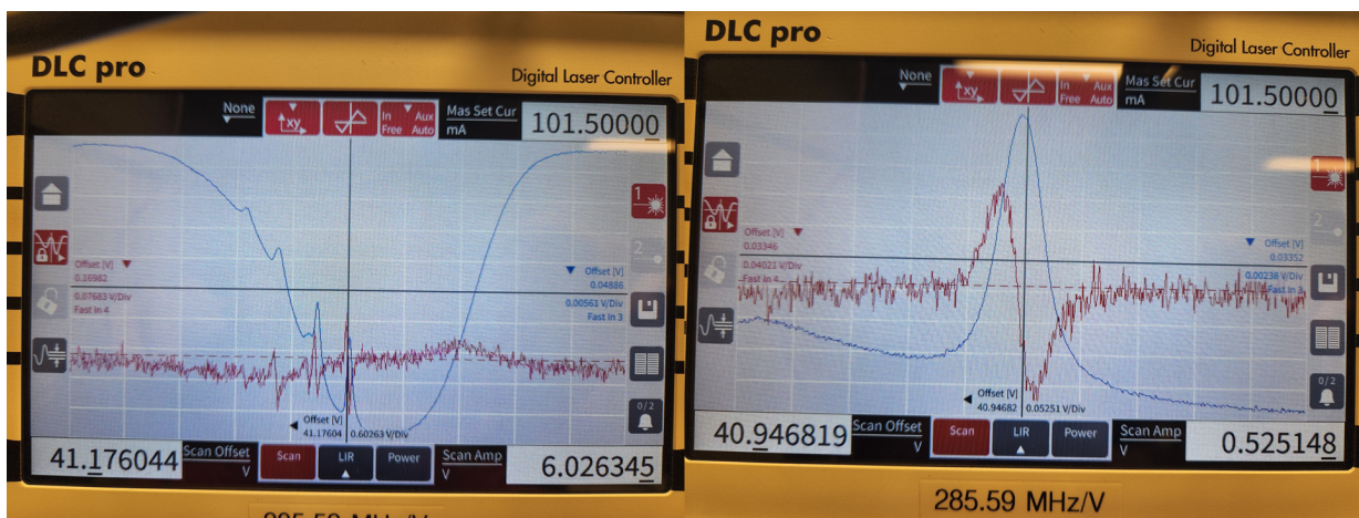
Figure 3.7: Oscilloscope trace of saturated absorption and FM spectroscopy.
