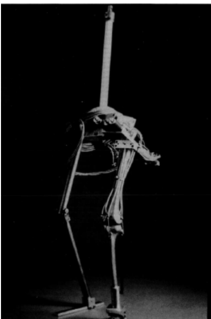
Figure 2.6: Surrogate leg tested in dynamic loading (Adapted from Paulos et al. (1991) )
