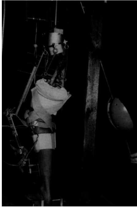
Figure 2.7: Cadaver leg being hit by a pendulum load (Adapted from Baker et al. (1989) )
