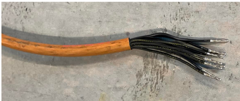
Figure 2.4: Cross-Section of 9/C EPR OKO Cable
