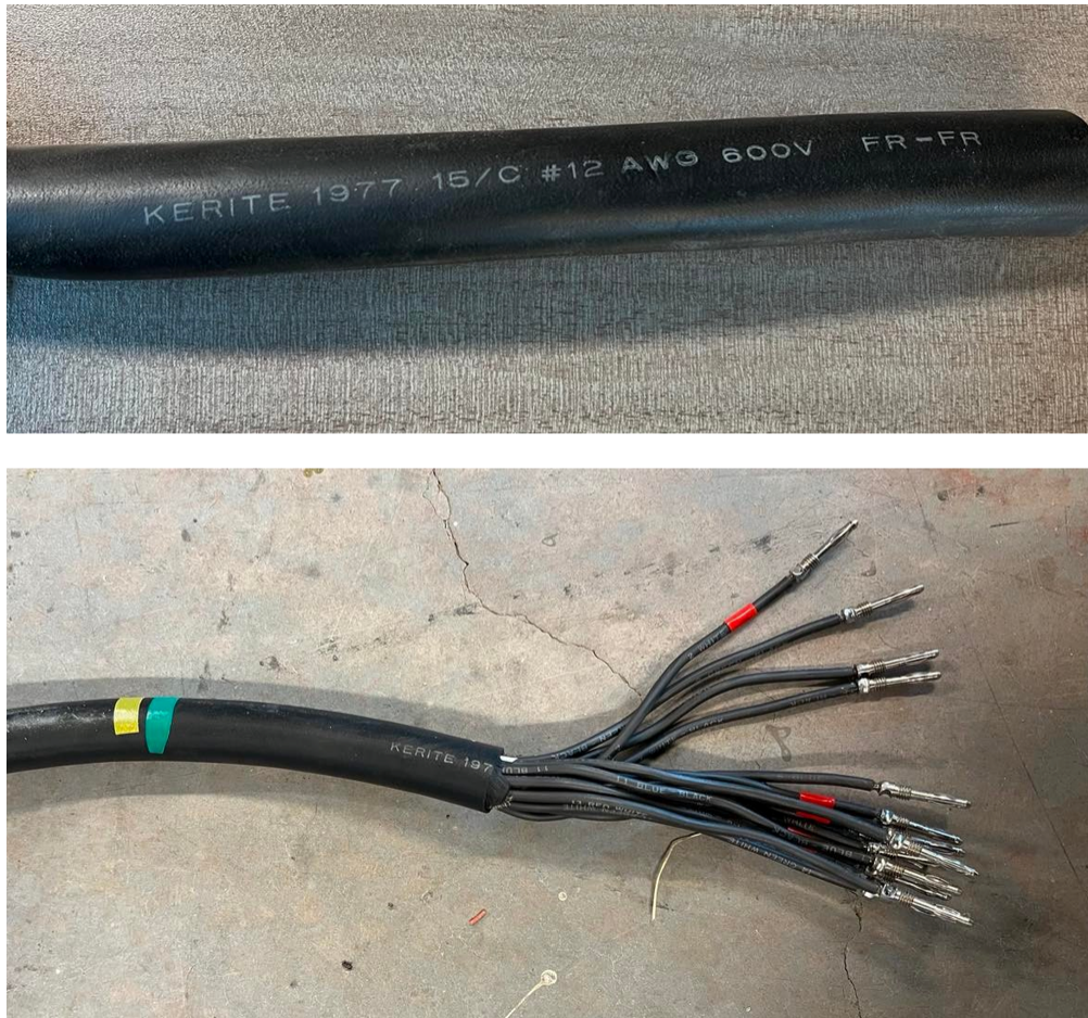
Figure 2.5: Cross-Section of 15/C EPR KER Cable
