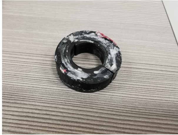
Figure 2.11: A 3D printed Plastic Part. It was used for wrapping the coils to act as barrier for a more natural transition from one layer to the next.
