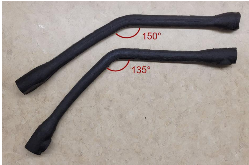
Fig. 4.4. The tortuous phantoms casted after two freeze-thaw cycles. Top: 30° phantom. Bottom: 45° phantom.
