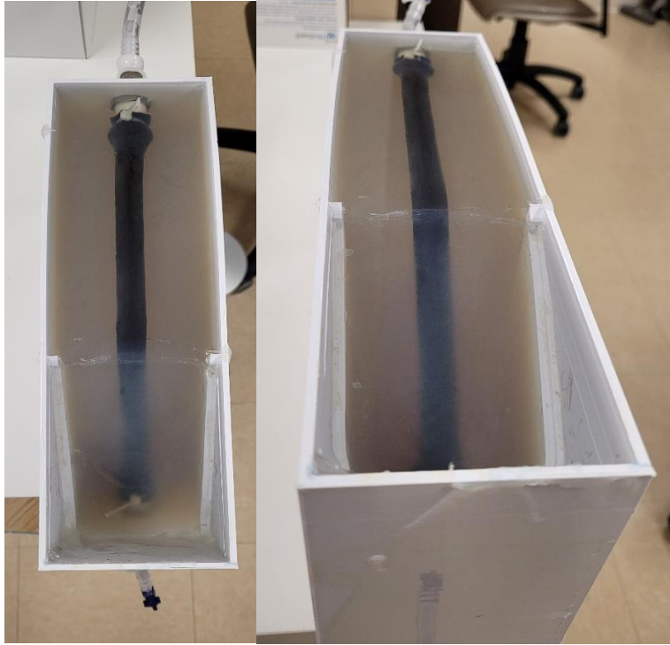
Fig. 4.6. Imaging box with slanted cover removed showing prostatic tissue mimic slab casted over the collapsed phantom.
