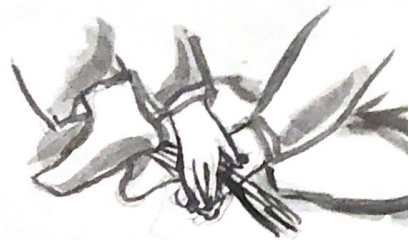
Pull after twisting to tighten the rope
