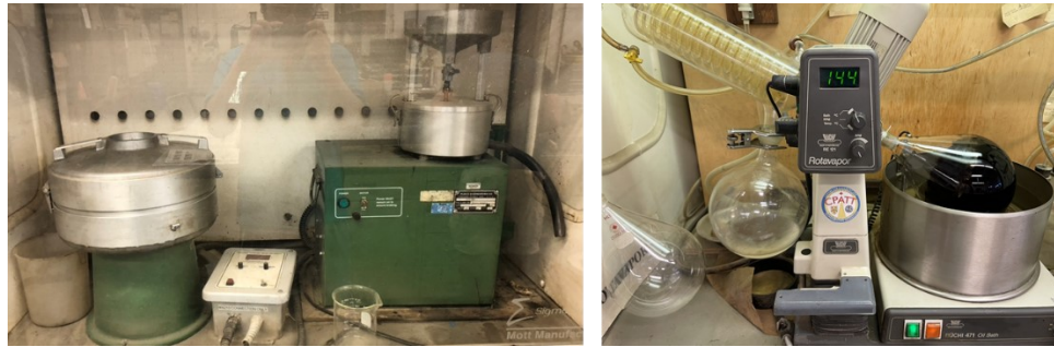
Figure 3.4 Centrifuge extraction and rotavapor recovery setup
