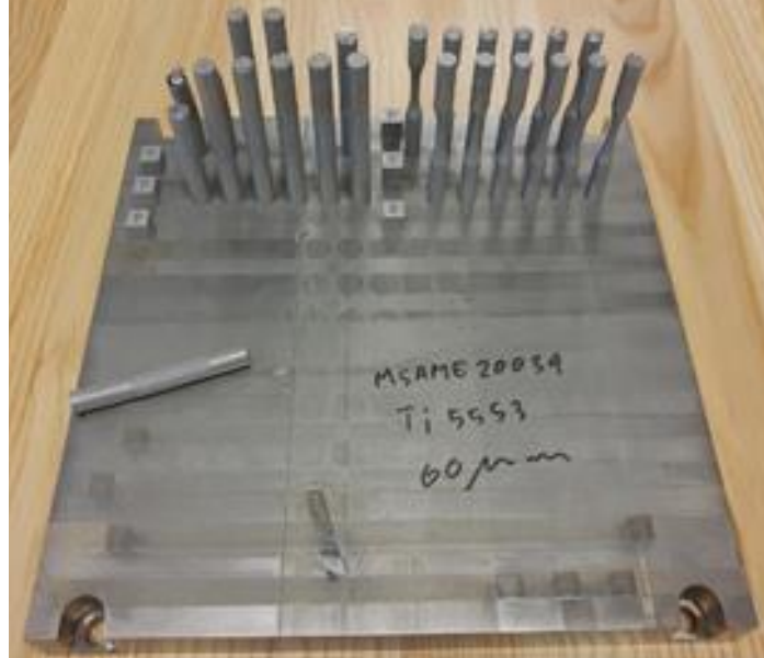
Figure 3-2: LPBF printed Ti-5553 samples on SS316 substrate plate
