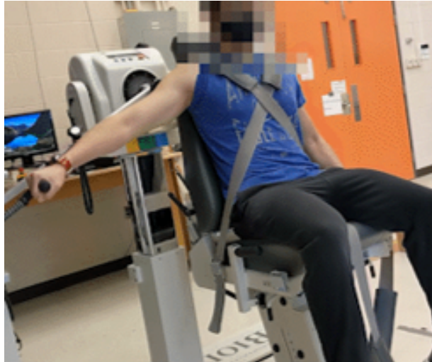
Figure 4.1: Example of a participant setup when \theta_1 is 0 deg and \theta_2 is 85 deg for isometric testing in elevation
