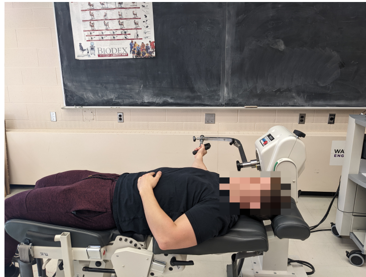
Figure 4.2: Example of a participant setup when \theta_1 is 0 deg and \theta_2 is 85 deg for the plane of elevation isometric testing.
